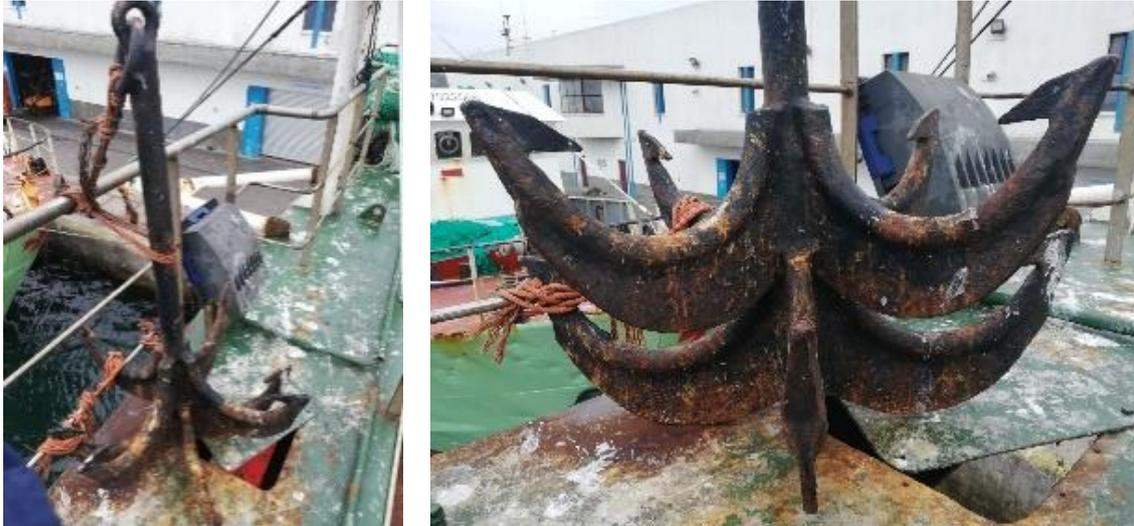
**Figure 4.** “Ressega” or “garateia”, tool used by fishers to recover lost gear on trawler vessels.
